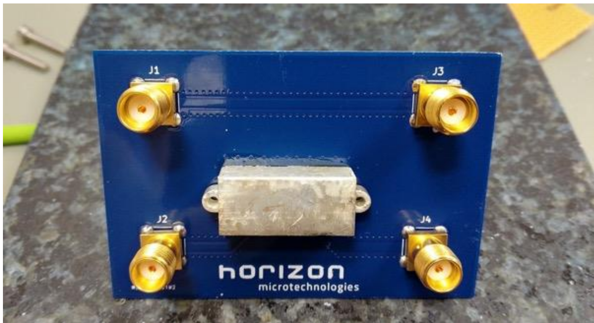
3D printed, silver coated polymer 5 GHz bandpass filter soldered to a PCB
