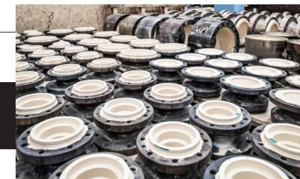
The application of the anticorrosive coating in all its phases is the most obvious work in a process that is made up of preliminary trials, tests and post-application checks. Powdered linings or liquid-based coatings are macro categories of an ever-evolving world not only in terms of product performance and quality, but also in terms of the coating process itself.
