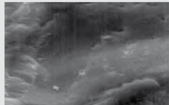
Cement with NovoCrete®: closed dense structure
