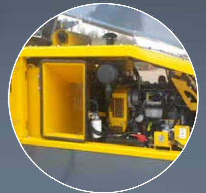
WIDE ACCESS ENGINE COMPARTMENT DOORS Provide perfect access for service and maintenance of engine and hydraulics.
