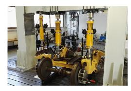
curve) as well as high-cycle fatigue properties (S-N curve, Smith chart) are tested, along with properties under multi-axial loading.
