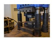
Other novel concepts include Q&P processing combined with incremental forming or forging. With a combination of novel techniques, components with strengths exceeding 1950 MPa and elongation levels of 15 % were produced.
