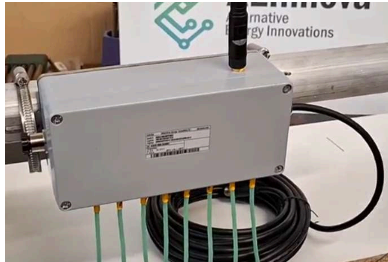
Batteryless IIOT device + 8 Thermocouples
