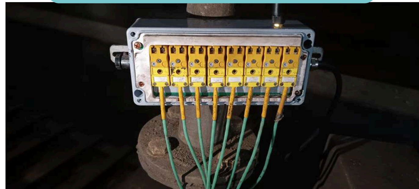
Batteryless IIOT device + 8 Thermocouples
