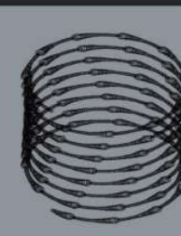
Figure 2: Printing path with a visible change in extrusion parameters
