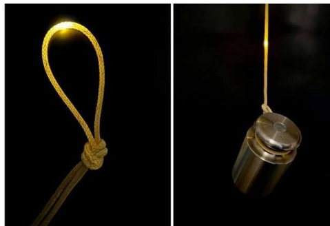
This single, elastic fiber contains a series of microdevices, including sensors, a microcontroller, digital memory, bluetooth modules, optical communications, and a battery, making up all the necessary components of a computer. An operating fiber computer shown knotted (left) and hanging with a 1-kilogram weight attached (right). (Courtesy Nikhil Gupta/Fink Lab MIT)
