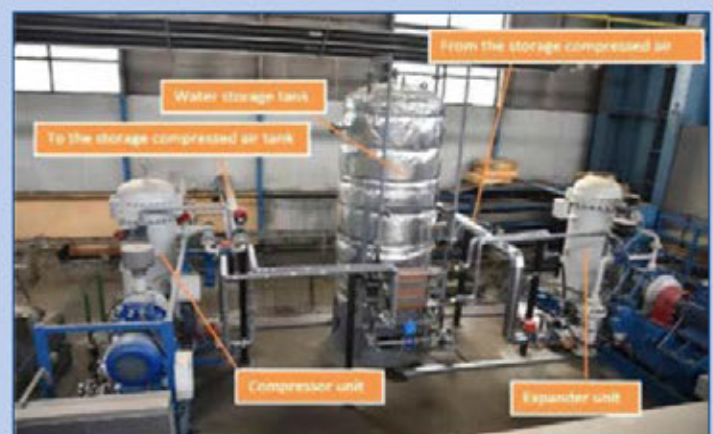
Pilot energy storage plant installed and commissioned at POPECI - Heavy Equipment, Craiova
