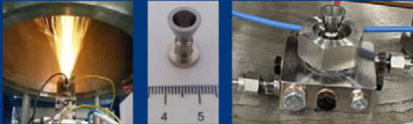
Green thruster based on water electrolysis, for AOC manoeuvres
