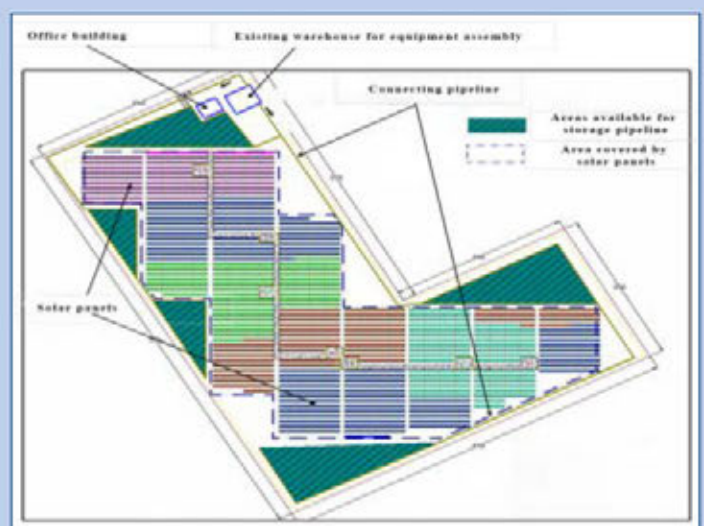
The plan for a photovoltaic power plant that uses CAES systems for energy storage
