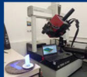
LC15Dx CMM automatic laser scanner, 1.9µm accuracy/ 22µm resolution
