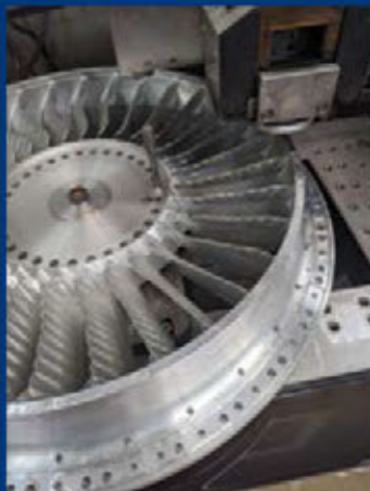
1/3 scale 3D printed OGV prototypes aero-acoustically tested
