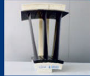
Triplet OGV mounted on a 3D printed stator case section
