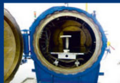
Autoclave - Scholz Ø1500 mm; length 2500 mm max. 400°C; max.20 bar; 6 vacuum lines/
