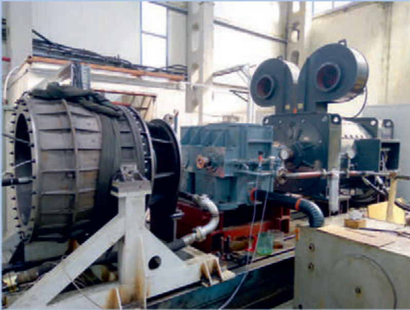
1.3 MW test rig with two stage, non intercooled MTI 1,500 compressor.
