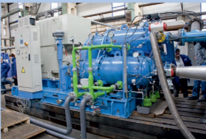
Compressor CCAE 9-125 (intercooled) on the test rig.
