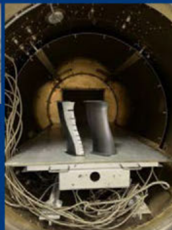
1/3 scale 3D printed OGV prototypes aero-acoustically tested
