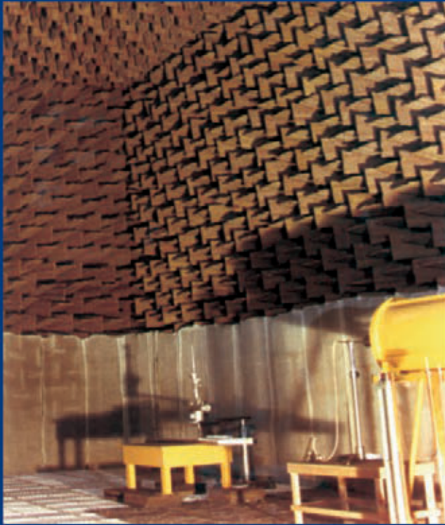
Acoustic tests - Anechoic chamber (1,200 m 3 ).
