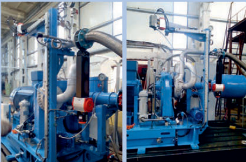
The arrangement of two other centrifugal compressors, with and without intercooling on the other test rig.
