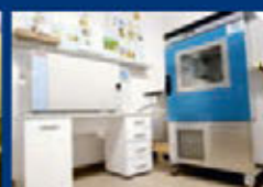
Environmental chamber Temp. range: -40°C up to +190°C/ CryoFreezer -140°C
