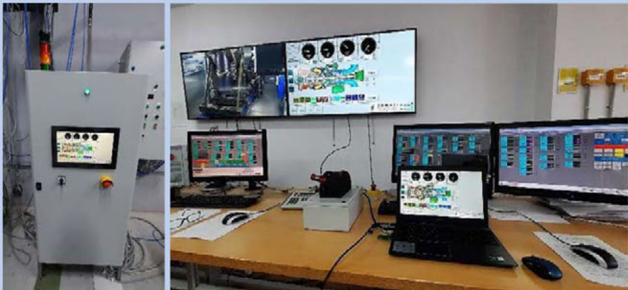
Automation system designed for testing ST40M marine gas turbine engines
