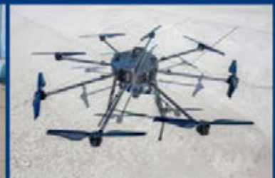
CFRP composite structure for Octocopter UAV equipped with hybrid propulsion solution
