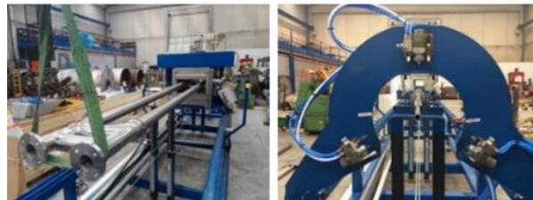
Automated coating line for pipelines
