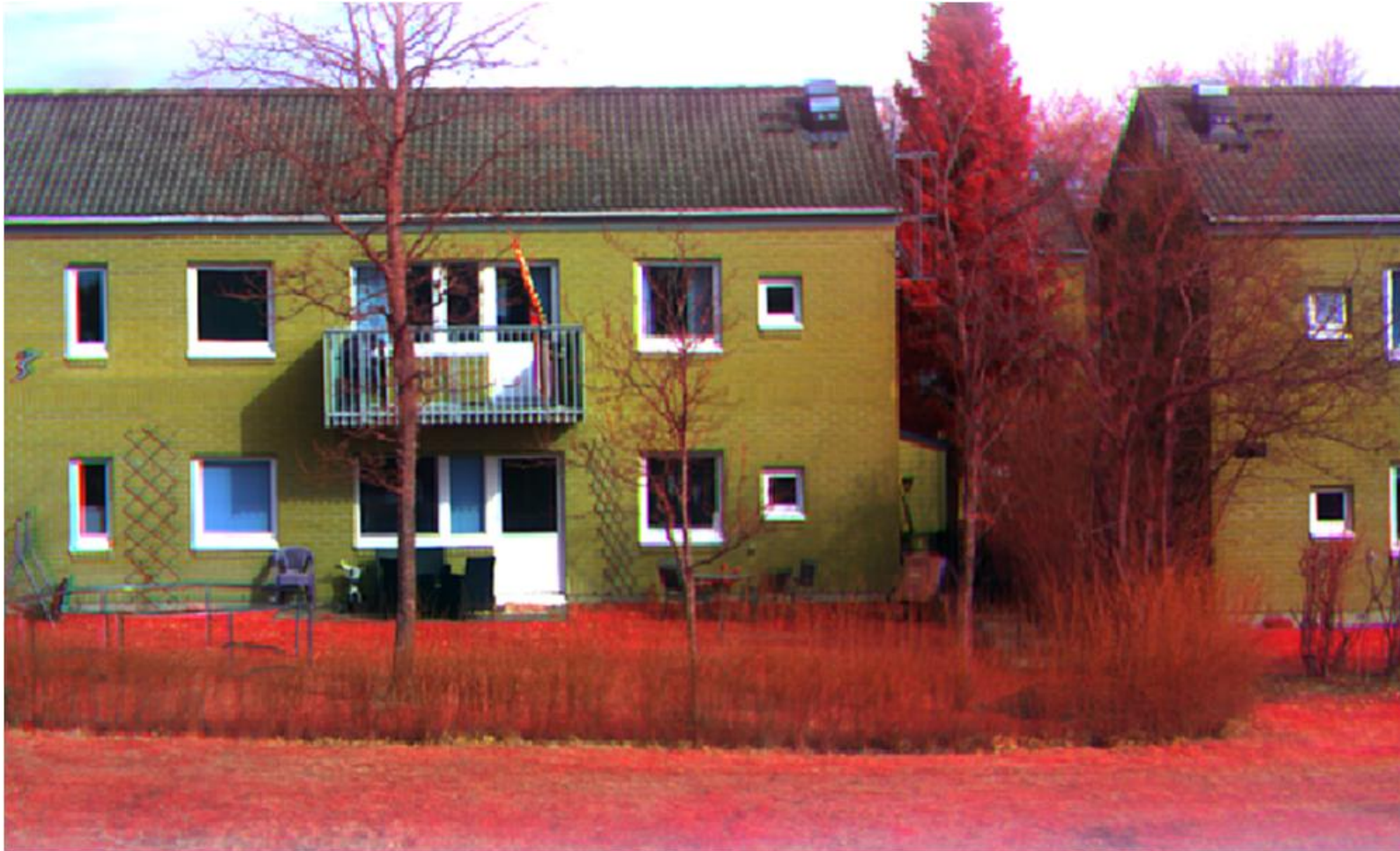
Hyperspectral scene shown in false colors, red→800 nm, green→650 nm, and blue→510 nm.
