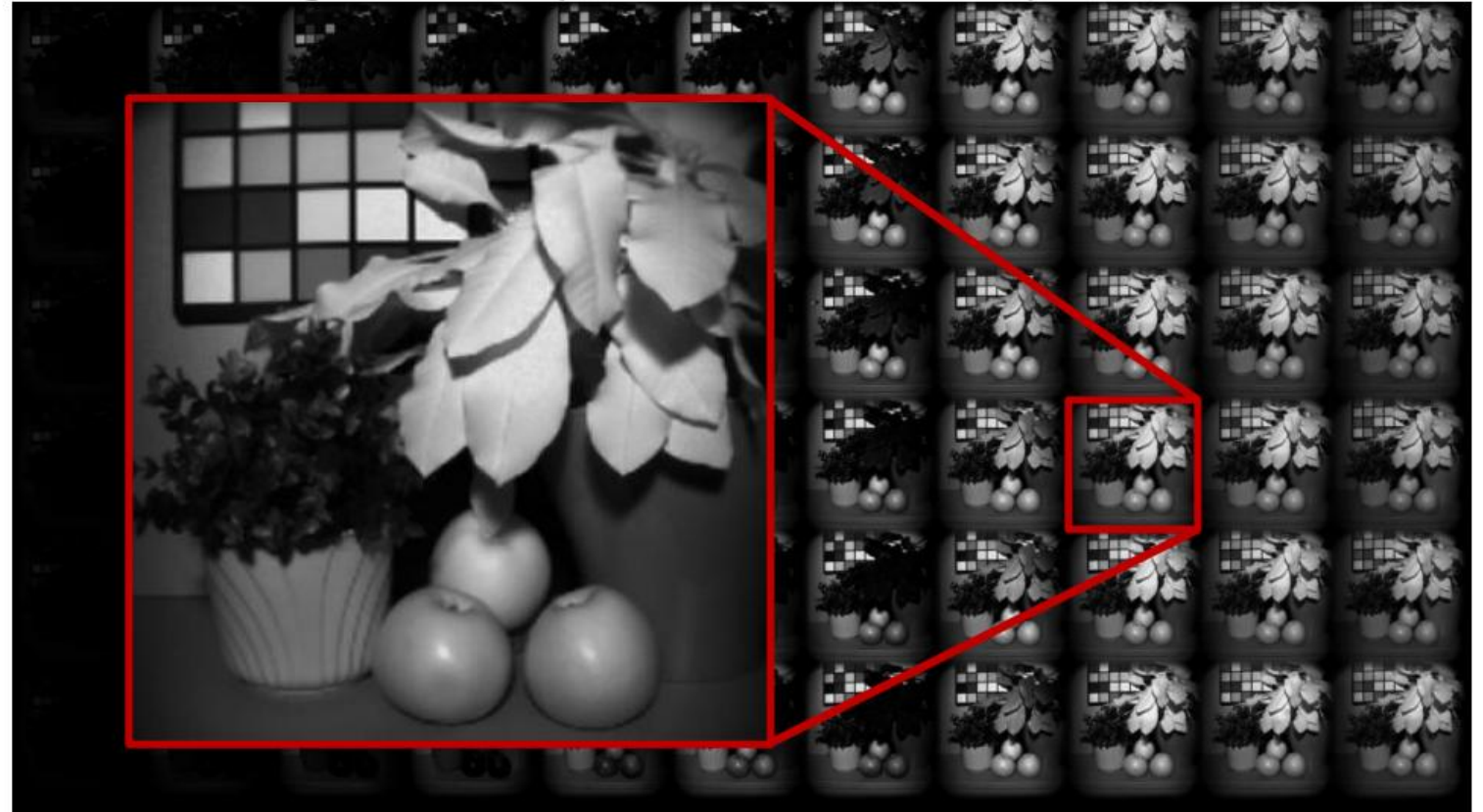
Raw image of Multispectral camera: 11x6 spectral channels
