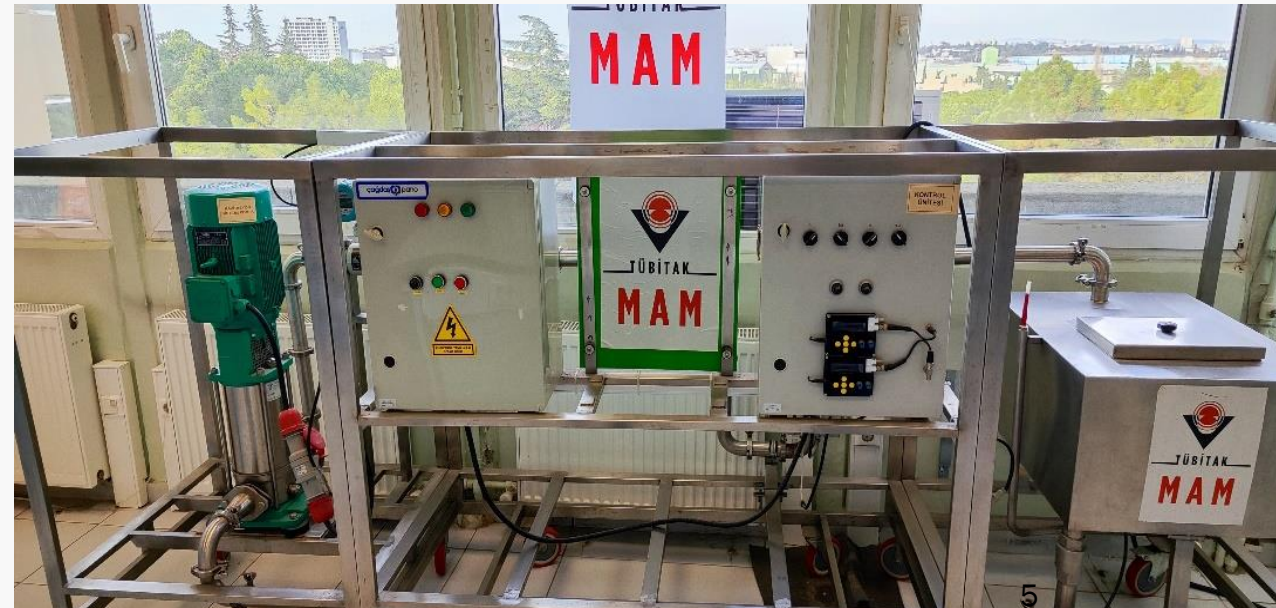
Hybrid cavitation reactor developed by TUBITAK MRC – patented technology
