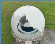
Innovative cylindrical non-rotating antenna and radar system
