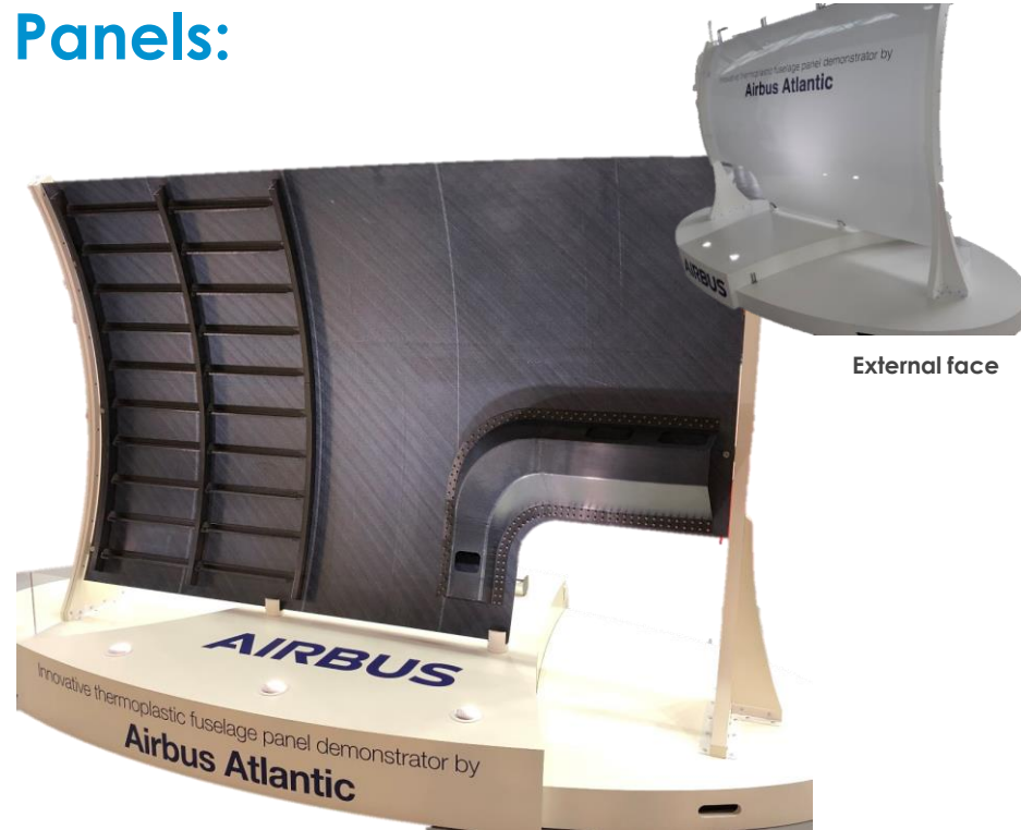
Welding of Z stiffeners on representative fuselage skin Welding study + demonstrator (Airbus Atlantic)
