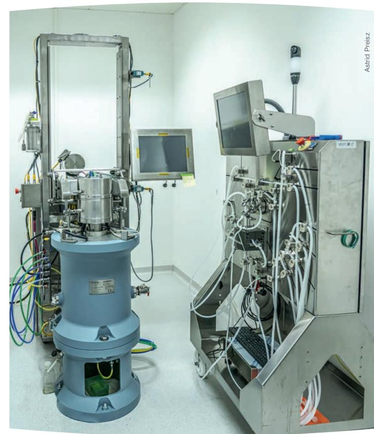
**Continuous ultracentrifuge pilot scale** (Alfa Wassermann pKII) with **fluid handling system** (Alfa Wassermann AFH)
