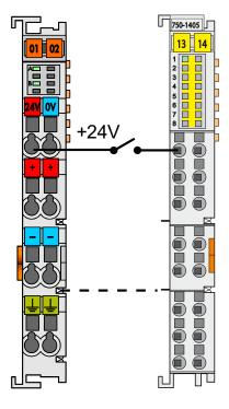
Dashed line is via PLC internal bus.
