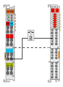
The dashed line is connected via the PLC internal bus.
