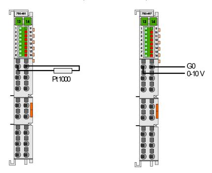
Operational readiness and trouble-free data bus communication of each input is **indicated** by green LED. For the 750-497 module, red LED indicates when measuring range is exceeded or falls below its limit for a given input. For the 750-451 module, red LED indicates wire break, short circuit or when signal is out of measuring range.
