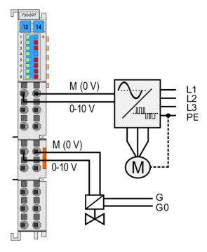
Operational readiness and trouble-free data bus communication of each channel is **indicated** by green LED. Red LED indicates status of the field power supply voltage (undervoltage or general error).
