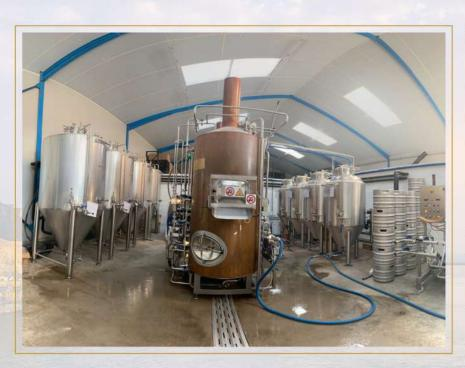
The A R G W E N beer is produced on site thanks to this production unit. After a day of brewing, three weeks follow in high fermentation in stainless steel tanks, Maison Jouffe has 8 (4 tanks of 600 liters and 4 tanks of 1200 liters). The annual production capacity is 100,000 L.
