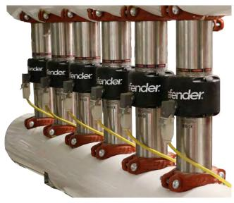
CSIDefender® chamber cells include "end-to-end" bi-directional internal laminar flow hydro dynamic features (8) that channels the water with less than 3PSI drop in pressure. This same feature prevents premature physical electrode erosion when installed in recirculated water loops and also offers reduced internal water turbulence and unwanted sedimentation deposits due to water eddies.
