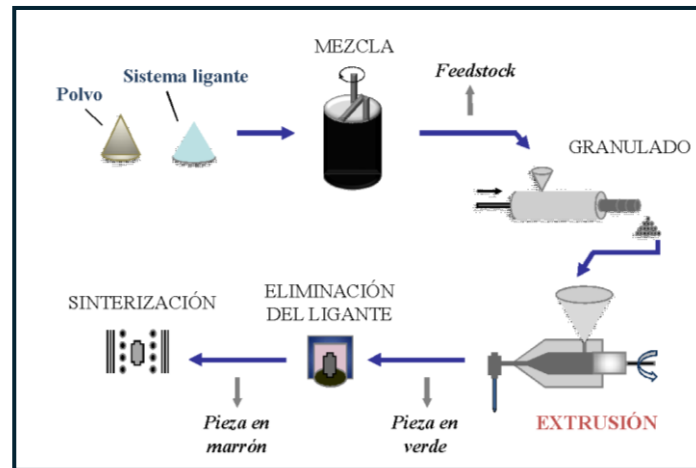
Schematic representation of the powder extrusion moulding (PEM) process
