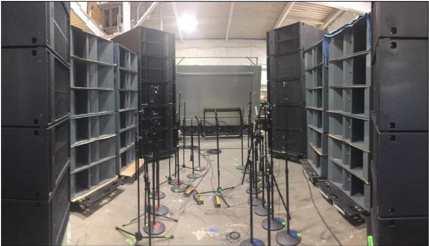
Small Satellite and Subsystem Test Setup to 3.6m tall.
