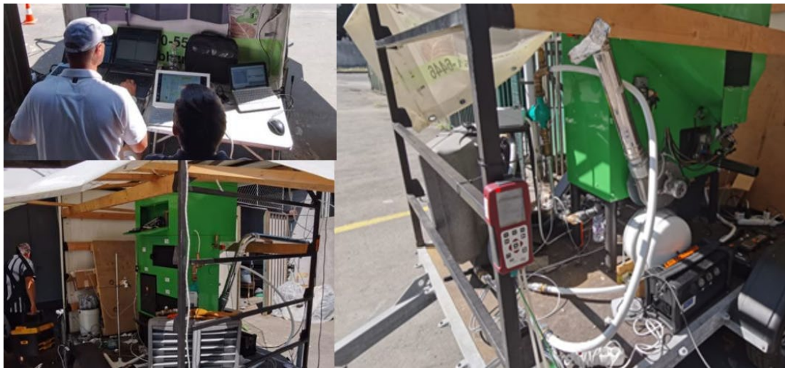
Automatic pellet boiler with catalytic infrared gasifier.
