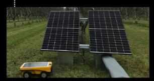
The solar panel mounted on top of VITIROVER allows the robot to work up to 6 hours a day, depending on the sunshine.
