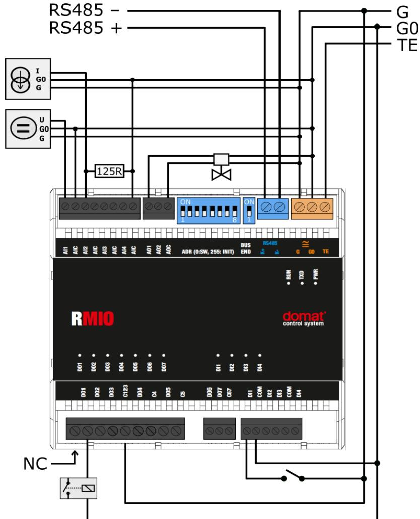
Analog inputs AI1 and AI2 have adjustable measuring ranges by jumpers facing the inner side of analog input terminals. AI3 and AI4 inputs have a fixed range (R, temp):
