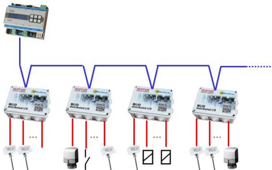
Together with the MLIO modules, there may be other module types on the bus, room units, variable speed drives etc., communicating Modbus RTU. However, separate buses for modules installed in the cabinet and outside the cabinet are recommended: with a common bus for all modules and short-circuit of the bus in the field, the communication with the modules in the cabinet would be broken.
