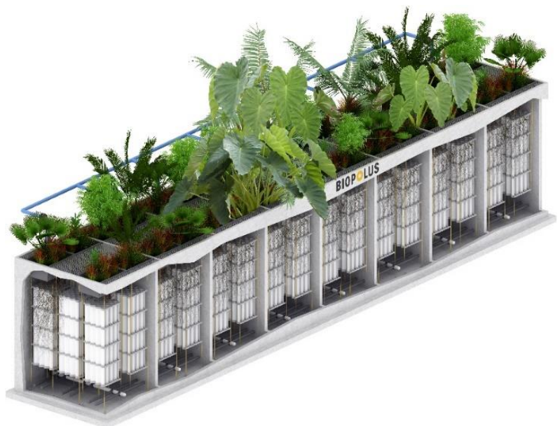
Figure 2. MNR biological water treatment uses natural & synthetic plant roots to provide optimal surface area for attached biofilm microbial growth.
