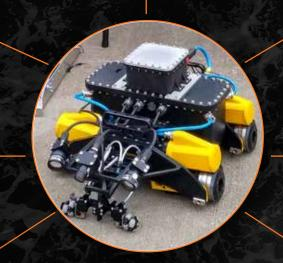
The rugged waterproof design ensures reliable operation in harsh marine and industrial environments, including in saltwater
