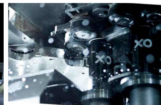
Seaming process can body/XO System
