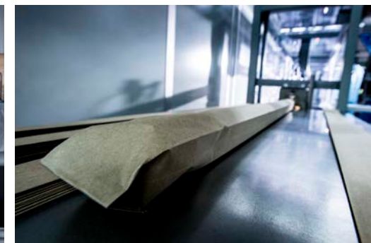
Packaging of final XO Ends into paper sleeves
