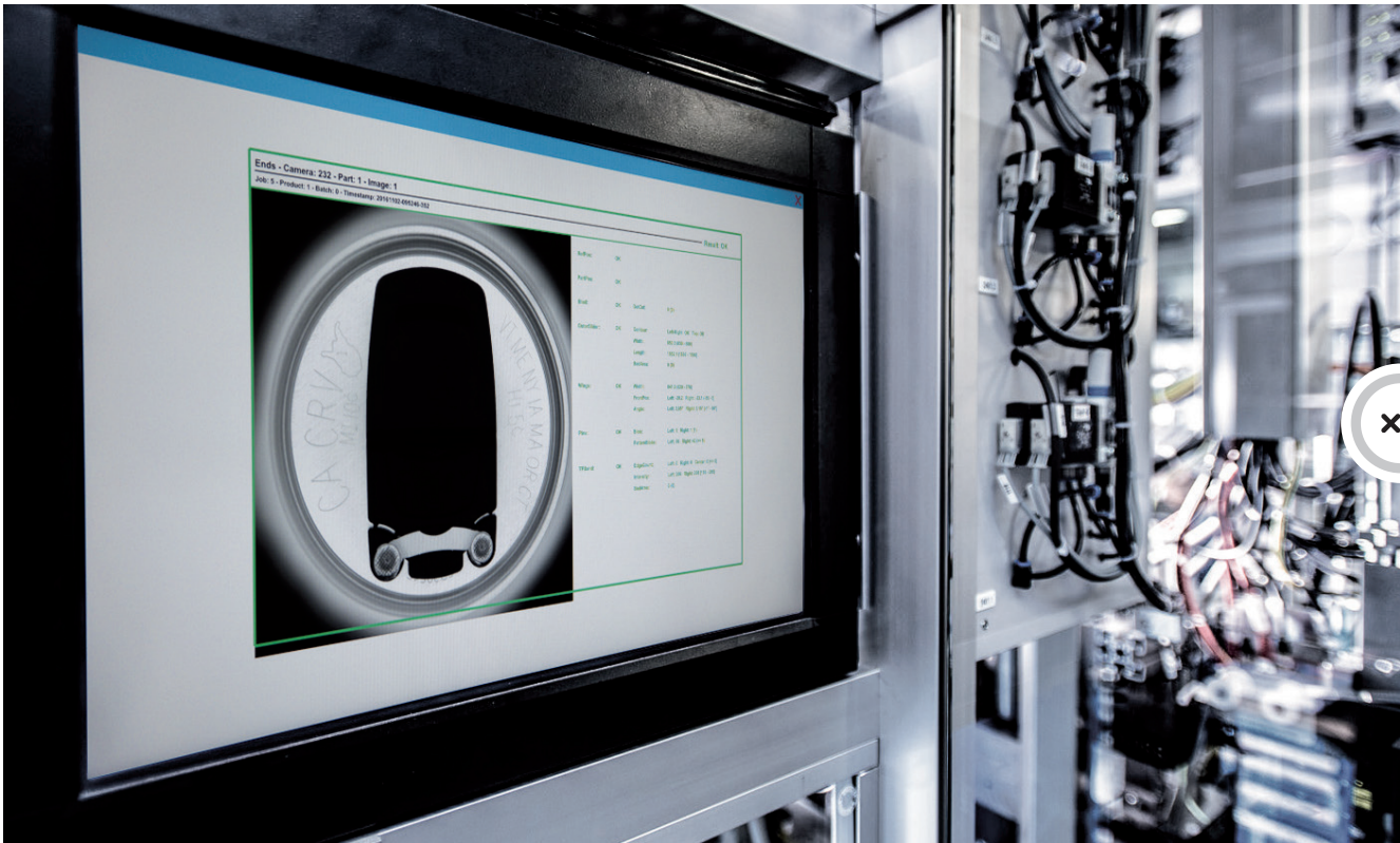
100% visual inspection of XO System
