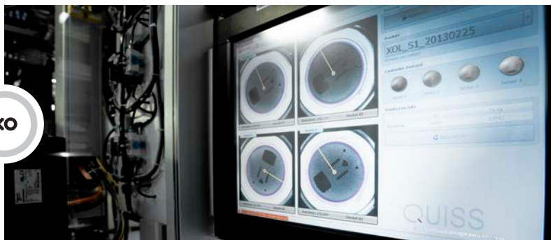
Visual inspection of shell
