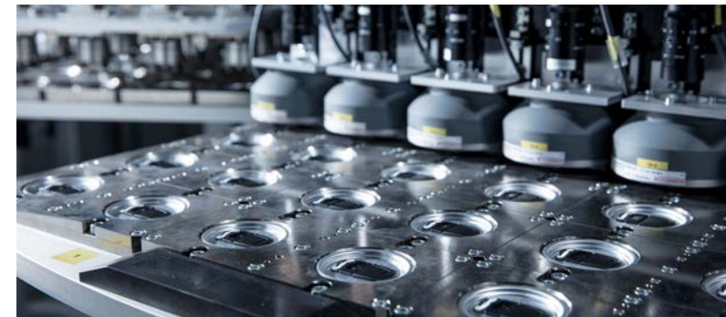
Visual inspection of finished ends
