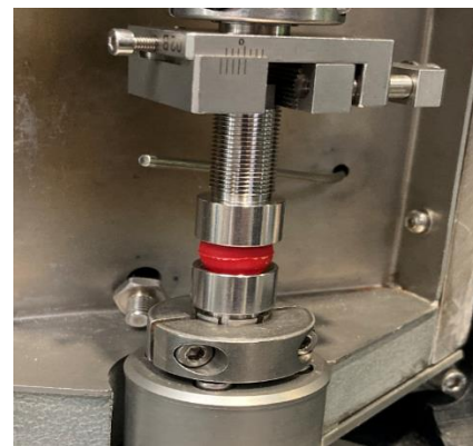
Figure 3: Compression Test Setup
