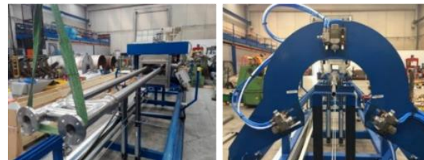
Automated coating line for pipelines
