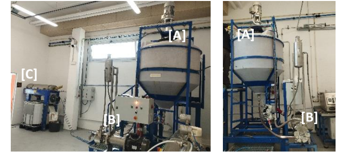
Pilot scale testing setup used to work at 200 L batches. ([A] 1000 L reactor, [B] homogeniser and [C] decanter setup)
