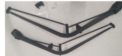
Windscreen wiper arm prototype FDM. ASA
