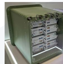
NEMUS Radar System Dimensions: 0,65 x 0,550x 0,38 meters
