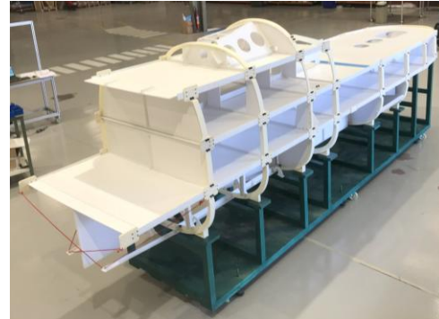
Jig for testing the assembly of equipment in the forward section of the EuroMALE/Eurodrone fuselage at a scale of 1:1 Dimensions: 6,50 x 1,35 x 1,35 meters
