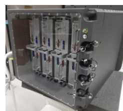
NEMUS Radar System Dimensions: 0,65 x 0,550x 0,38 meters
