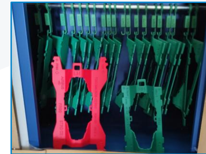
Part Shapes control jigs for stringers
