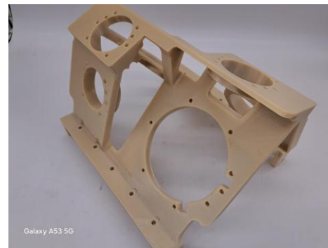
Multi-system support 280 x 160 x 230 mm. FDM. Ultem 9085
