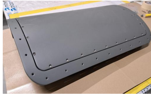
Antenna SATCOM AESA Dimensions: 0,58 x 0,41 x 0,15 meters
