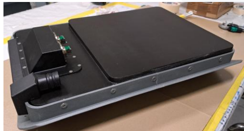
Antenna SATCOM AESA Dimensions: 0,58 x 0,41 x 0,15 meters
