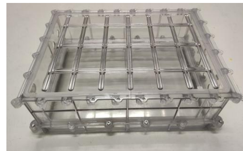
Transparent box to house electrical circuitry Dimensions: 0,50 x 0,37 x 0,20 meters
