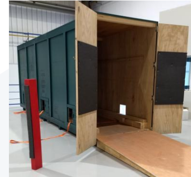
Jig for testing the assembly of equipment in the forward section of the EuroMALE/Eurodrone fuselage at a scale of 1:1 Dimensions: 6,50 x 1,35 x 1,35 meters
