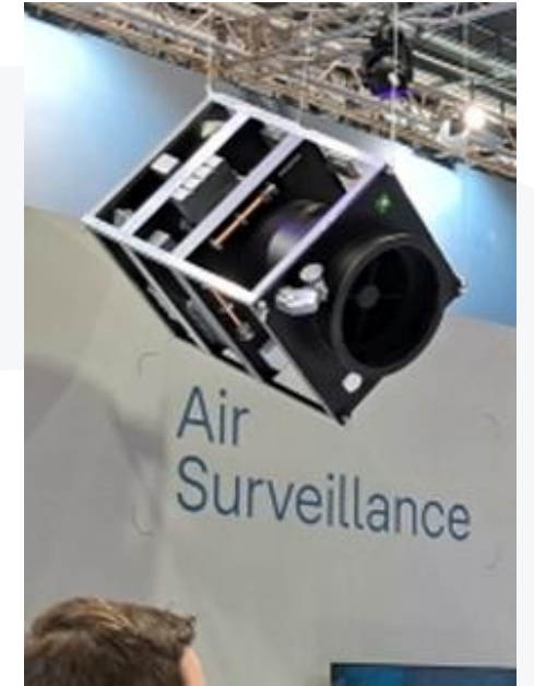
Mini4EEO satellite Dimensions: 0,60 x 0,60 x 1,00 meters
