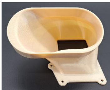
Air duct. 170 x 150 x 110 mm. FDM. Ultem 9085
