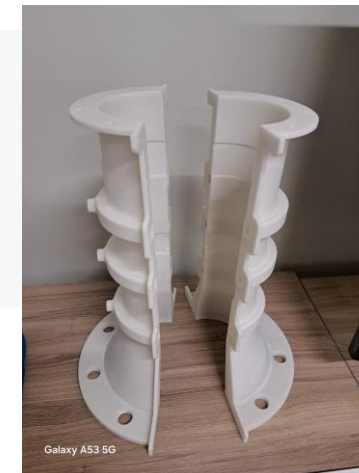
Prototype flanges D410 x 310 mm. SLS. PA12
