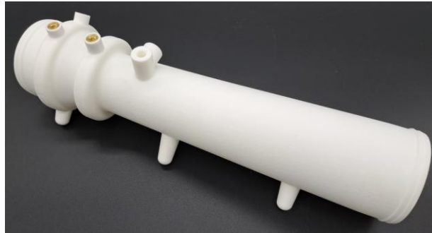
Laboratory Flow meter 90 x 90 x 300 mm. SLS. PA12
