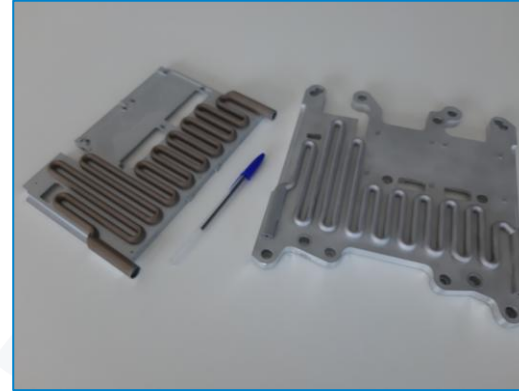
Cooling plates for electronic circuits. DMLS (Hybrid manufacturing). AlSi10Mg
