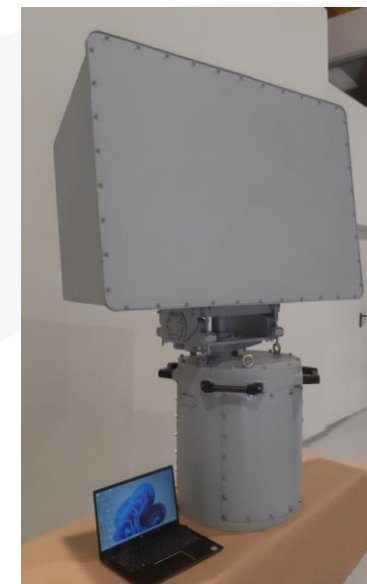
Naval Antenna 1,50 x 1,15 x 0,95 meters Weight: 130 kg
