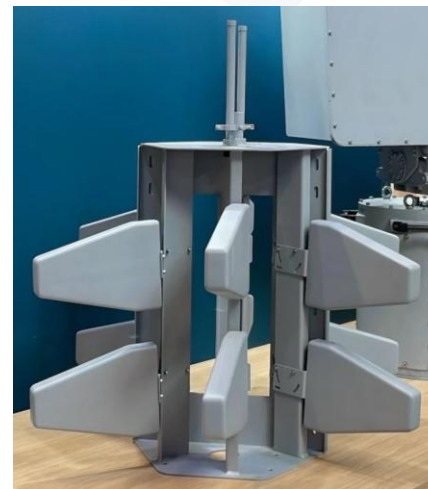
Jammer antenna sets (x2) Dim: 0,60 x 1,00 x 1,10 meters
