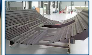
Part Shapes control jigs for stringers
