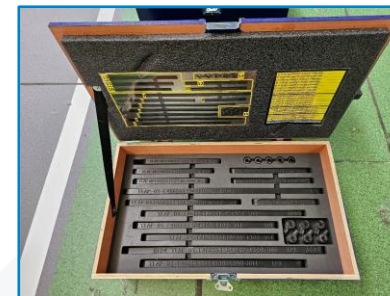
Drilling template storage boxes at Airbus plant.
