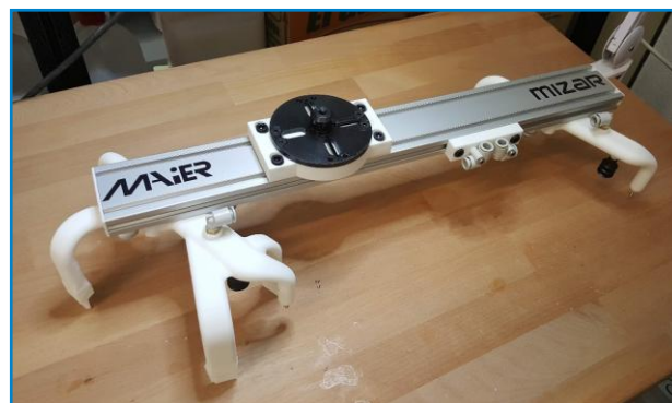
Robot grippers for transferring parts in a plastic injection moulding process. FDM. ABS/ASA
