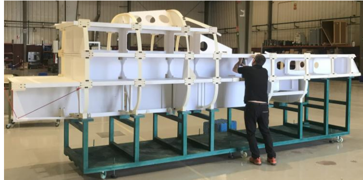
Jig for testing the assembly of equipment in the forward section of the EuroMALE/Eurodrone fuselage at a scale of 1:1 Dimensions: 6,50 x 1,35 x 1,35 meters
