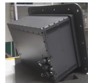
NEMUS Radar System Dimensions: 0,65 x 0,550x 0,38 meters
