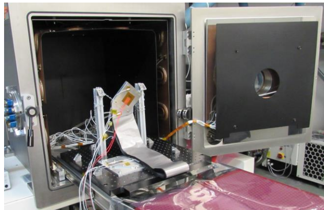
MTVAC Thermal conductance test (in-house)
