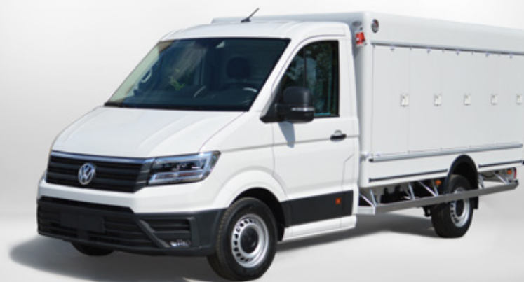
Refrigerated truck with eutectic cooling
