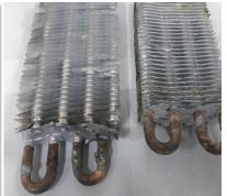
Catholic corrosion protection solution of **aluminum nitrate (AlN) film** as an **anticorrosive coating** in metallic Heat Exchangers (HE) components, against corrosive conditions including salt hydrates PCMs.
