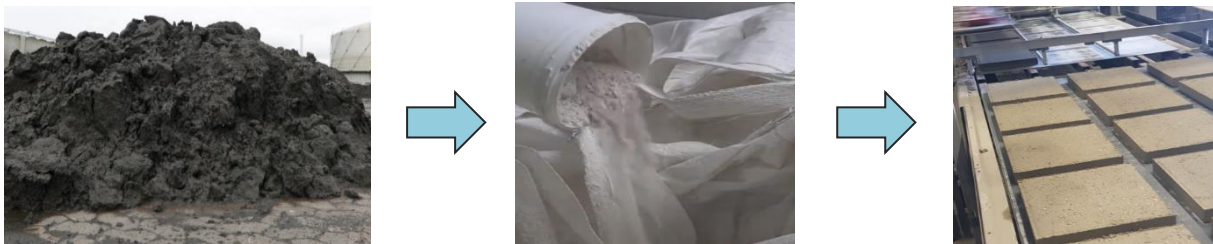
Figure 1: The MID MIX process converts sludge (left) into Neutral (middle) which has multiple applications, such as use in pavement slabs (right)
