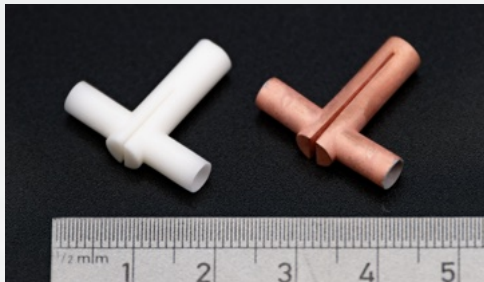
3D printing and metallization of ceramics also enables dielectrically loaded devices such as this orthomode transducer
