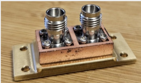
Combination of 3D printed and machined parts in splitblock-type design, and connectors/adapters opens additional design possibilities
