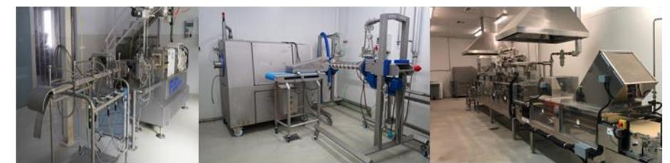
Dry/HME/cooking extrusion: 4x pilot extruders
