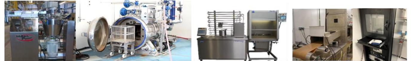
Formulator | Autoclave | UHT lane and aseptic packaging | Microwave treatment. | Cold plasma
