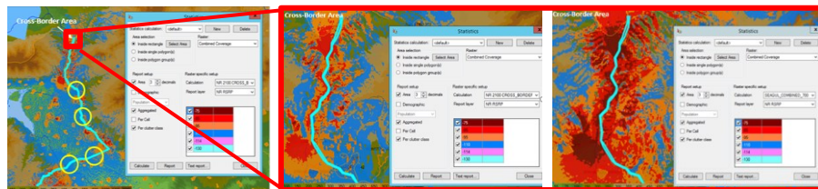
COSMOTE 2100MHz COSMOTE predicted coverage in GR/ Serres segment of the CBC, depicting coverage gaps
