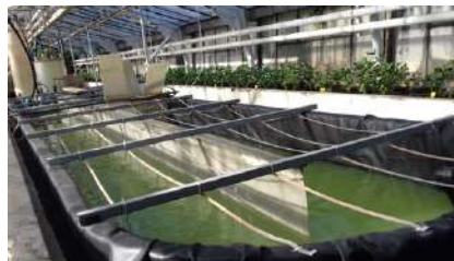
Microalgae cultivation raceway open pond, 10 m 3 – Complex project 32PCCDI/2018
