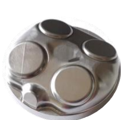
Component to repair (combustion chamber die) in H13 tool steel
