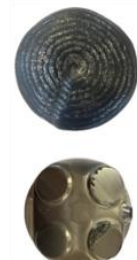
3. Deposition of material and finish milling to obtain the final result
