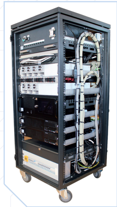
19" test cabinet for a radar surveillance system, complete mechanical construction and wiring with VDE testing and documentation
