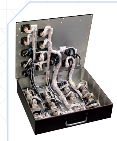
Wiring adapter for an engine test bench, electromechanical construction and wiring
