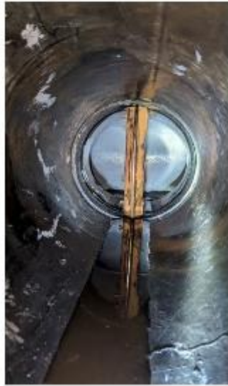
BALLAST PIPE IN ER STRENGTHENING USING ENECON PUTTY (Ceramalloy CP+AC)
