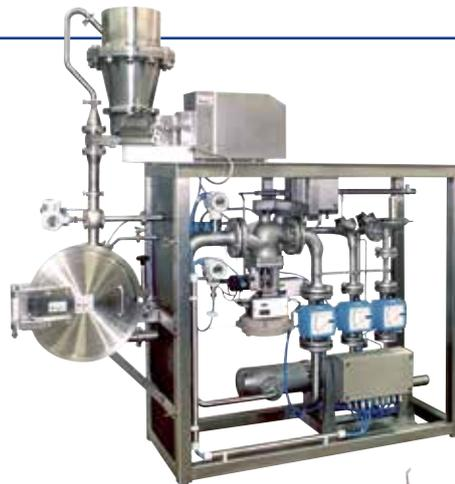
*315 AS module with PDD 30 double metering screw*
