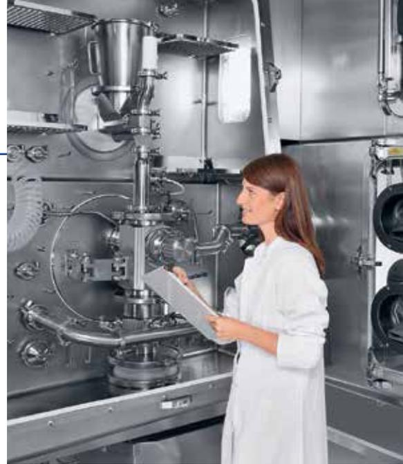
70 ZPS isolator solution with PDD 25 metering screw
