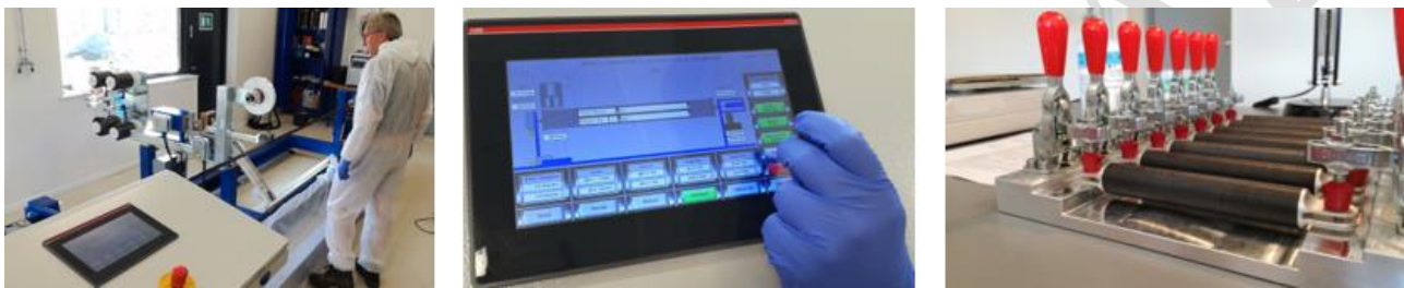
Figure 11 Inhouse manufacturing from left: Filament winding of CFRP tube, digital controlled CNC, struts in bonding jig
