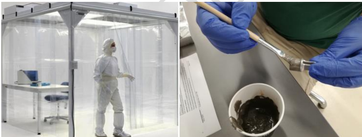
Figure 12 ISO 8 soft wall cleanroom (installed in October 2018), mainly for bonding, cleaning & contamination control purposes
