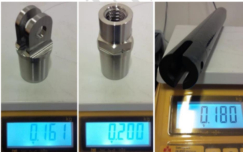
Figure 8 The whole strut has a mass of one equivalent INVAR metallic fitting
