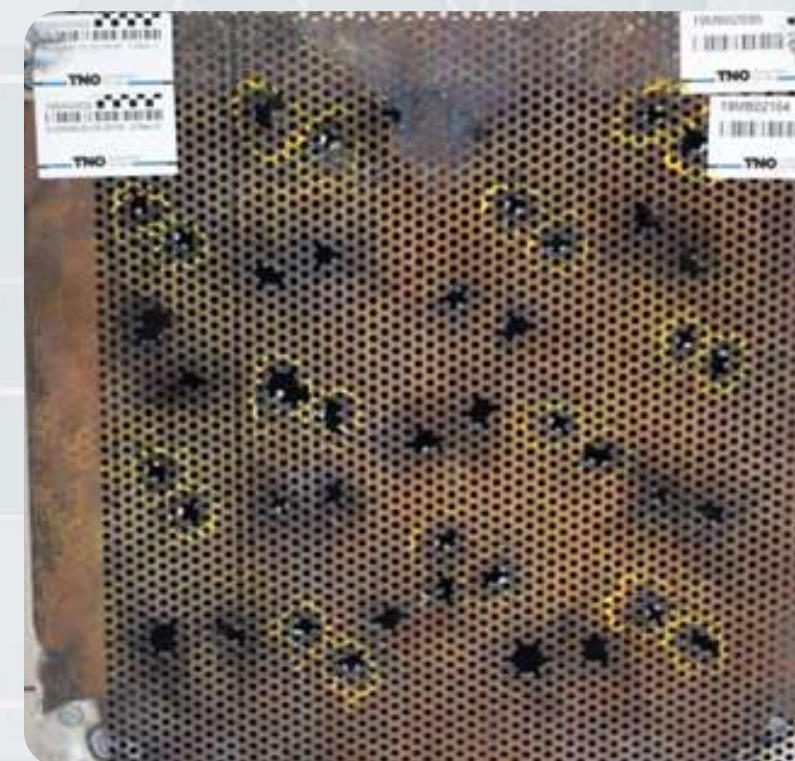
44 Shots on Single 500x500 mm Panel for Stanag 4569 Level 3
