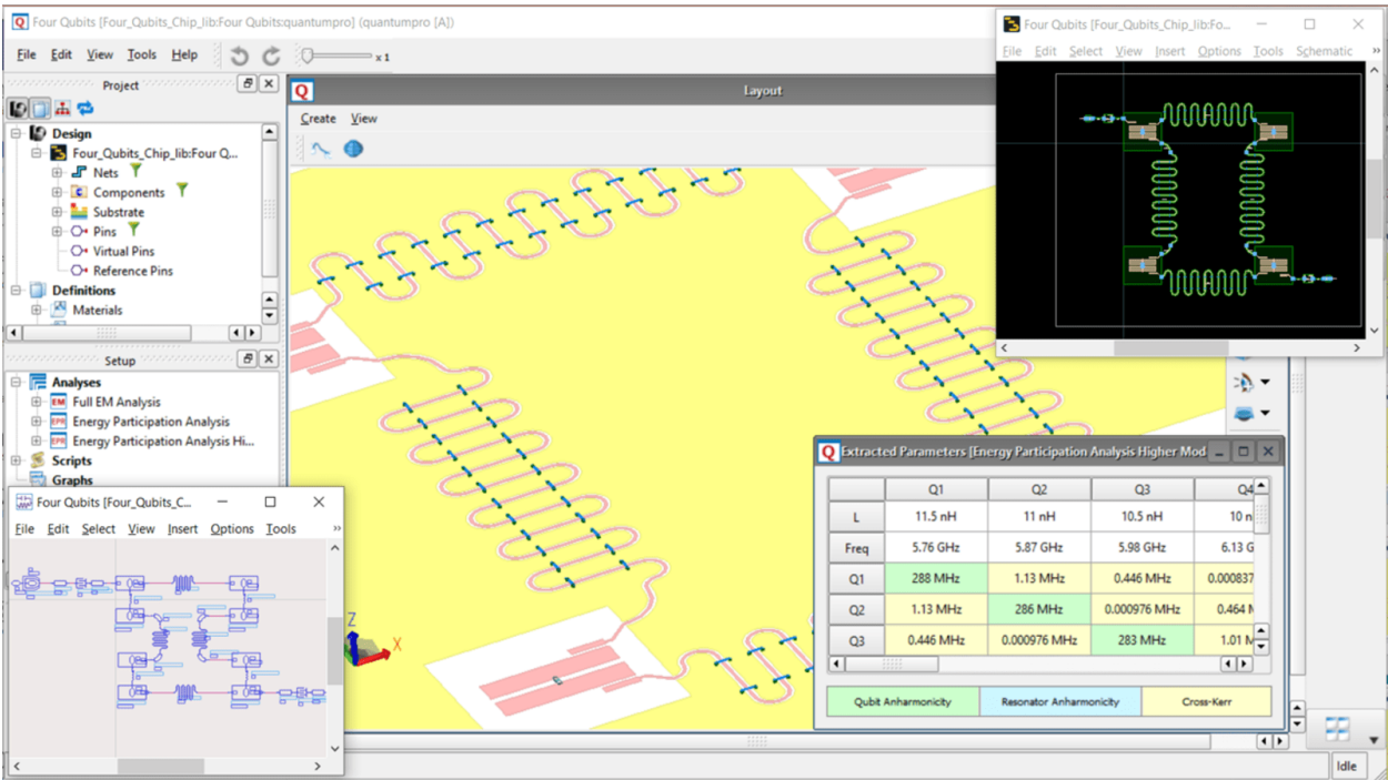
Figure 4. A four qubits circuit example in QuantumPro.
