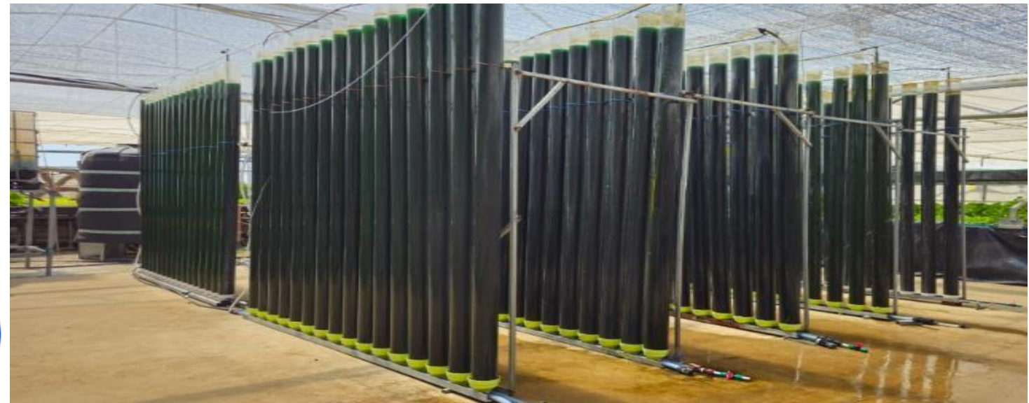
Automated remote-controlled PBR :
