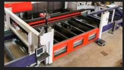
Laser cutting machine Bystronic Bystar 4025 Width up to 2500mm Lenght up to 6500mm Power 6kW
