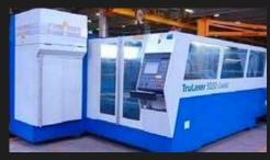
Laser cutting machine Trumpf TruLaser 5030 Classic Thickness up to 25mm Width up to 1500mm Length up to 3000mm Power 5000Wt
