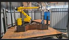
Welding robot Fanuc M710iC/12L Load capacity up to 12kg Reach up to 3123mm Axis robot 6
