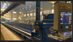
Gas/Plasma cutting & drilling machine MGM Omnicut MS300 Thickness up to 220mm Width up to 4m Lenght up to 27m Drilling up to 50mm
