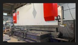
Press brake Bystronic PR400/6200 Thickness up to 15mm Length up to 6000mm Power 400tns
