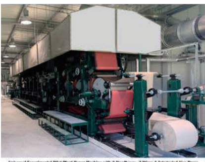
Universal Experimental Pilot Plant Paper Machine with 3 Headboxes, 2 Wires &amp; Integrated Size Press
