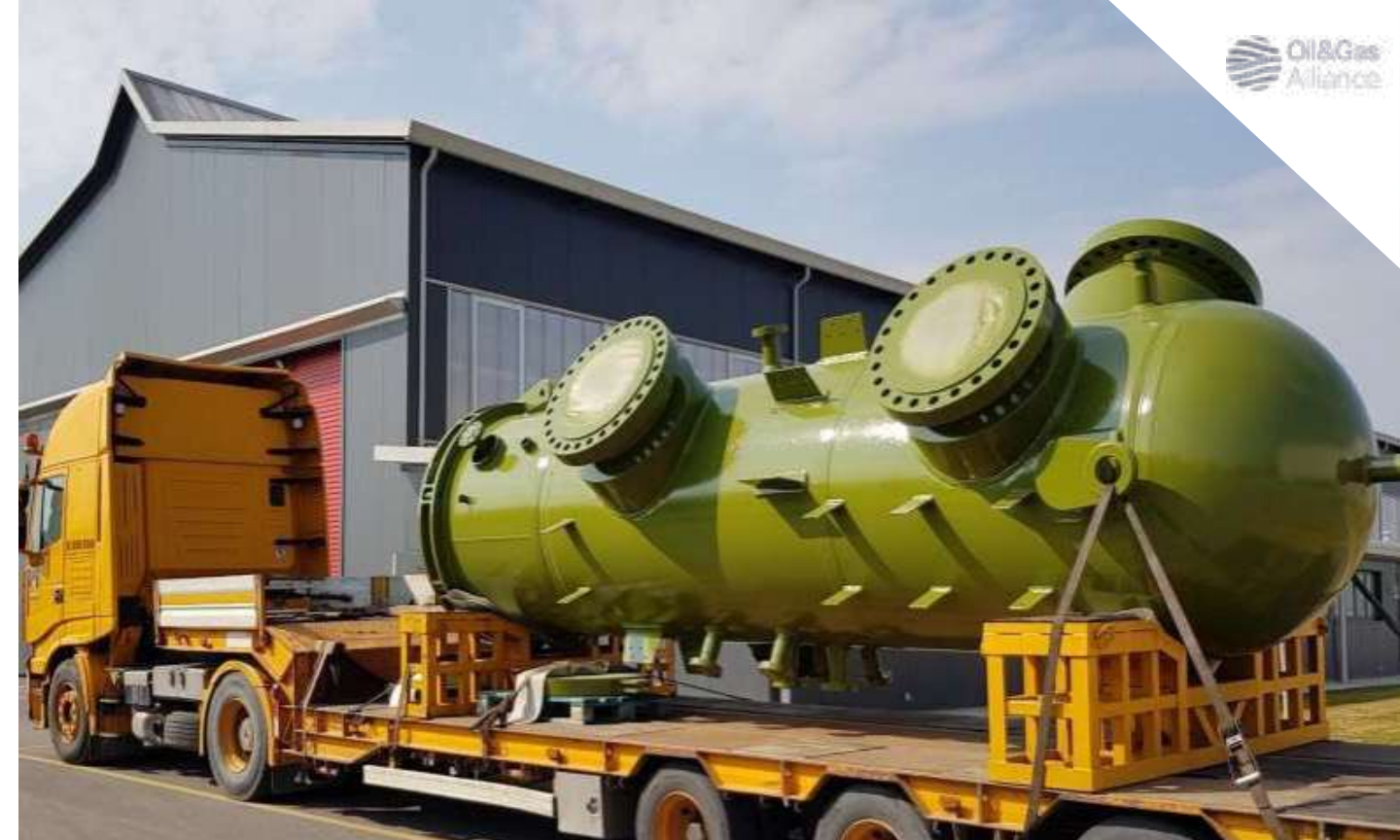
LG Coalescers + Platforms In SA-516 Gr.70, H = 6.700 mm, OD = 1600, Thk = 60 mm For Storengy – Stablack Gas Storage Project Phase II (UK)
