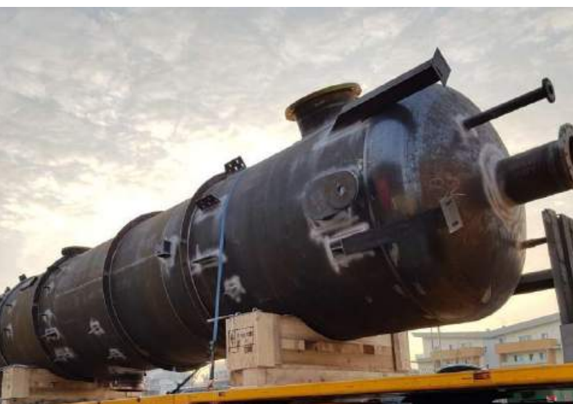
Gas Dehydration Inlet Coalescer + Platforms In SA-516 Gr.70 + Clad in SA-240 316L, H = 9.030 mm, OD = 2050, Thk = 72+2 mm For SNC Lavalin / Sonatrach - Rhourde Nouss Project (Algeria)
