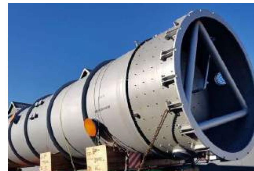
Nr. 1 Tail Gas Drum in SA-516 Gr.70, L = 30.000 mm, OD = 3.875 mm, Thk = 15 mm For UOP (process licensor)
