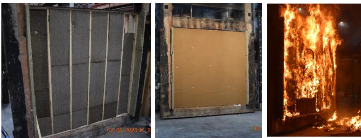
Figure 4: One of the tests done in project Wood Uphigh with seaweed wool insulated wood construction a) during the assembly prior the test b) after 67 min of test c) specimen seen from exposed side right after the test
