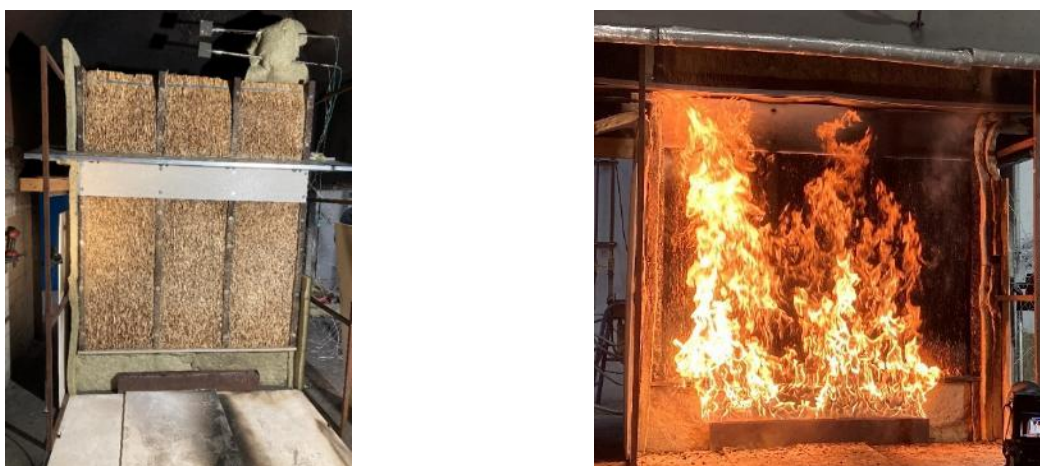
Figure 3 Intermediate scale tests of thatched façade/external wall construction and physical barrier for limiting fire spread.
