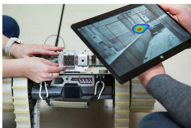
NANOPIX embedded on UGV in the framework of the European project TERRIFIC
